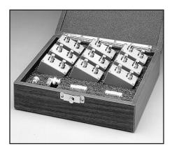
**Model 5905:** Calibration sources for Model 590/1M. Includes 18pF, 180pF, 1.8nF, 4.7pF, 47pF, 470pF capacitance sources and 180μS, 1.8mS, 18mS conductance sources. Also includes CS-566 right angle male-to-female BNC connector, CS-567 female BNC shorting cap, and 5900-313 storage case.
