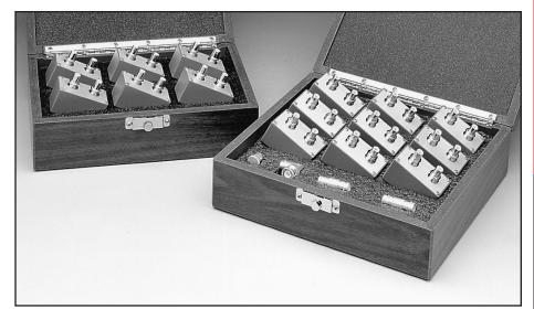
**Model 5906:** Calibration sources for Models 590/1M, 590/100k, 590/100k/1M, and 5904. Includes 1.5pF, 18pF, 18pF, 18nF, 0.5pF, 4.7pF, 47pF, 47pF, 4.7nF capacitance sources and 1.8μS, 18μS, 18μS, 18μS, 18mS conductance sources. Includes two storage cases.
